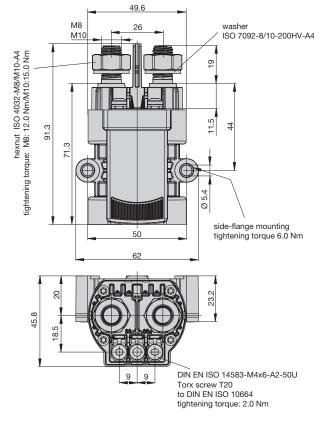
Mounting method 1 including option 4 – 3-pole connector compatible with Tyco HDSCS
