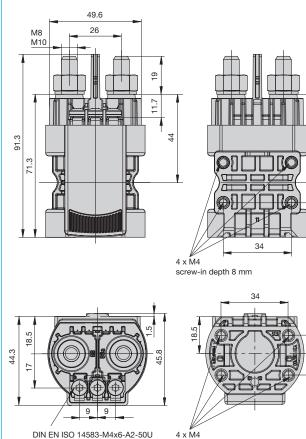
DIN EN ISO 14583-M4x6-A2-50U Six lobe screw T20 to DIN EN ISO 10664 Version with side flange (50 mm distance between holes) and M4 screw terminals
